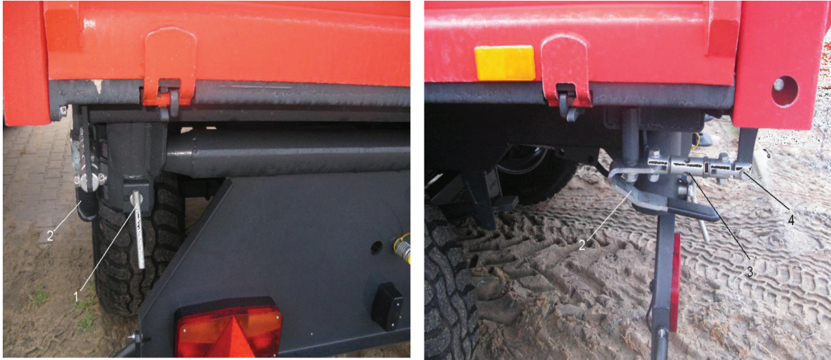
Fig. 5. Load body wall locks
